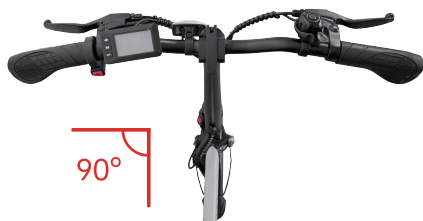
14. Check whether the handlebar is 90° perpendicular to the frame or front wheel.
