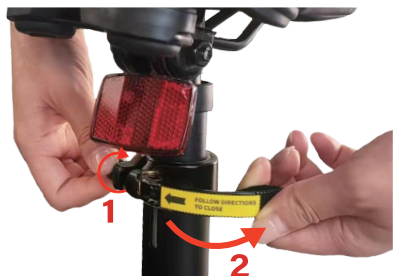
15. Put the seat post into the seat tube. Note: Do not raise the seat post to expose the minimum scale mark on the seat tube. Turn the knob on the seat post clamp to the appropriate tightness, then press the handle to lock it.
