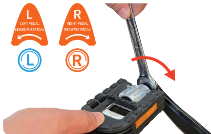
18. Find the pedal shaft and pedal marked with the corresponding letters, and tighten the nut in the direction indicated by the pedal shaft sticker.
