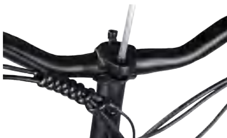
13. Tighten the handlebar quick release screws.
