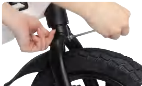
17. Install the front fender on the front fork. (When unboxing, the front fender and rear fender are tied together, please take off the front fender)
