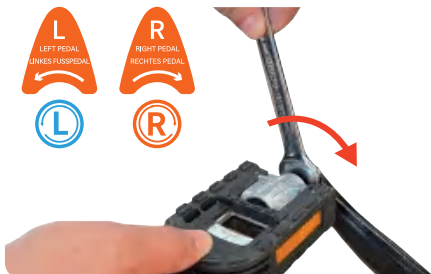
18. Find the pedal shaft and pedal marked with the corresponding letter, and tighten the nut in the direction indicated by the pedal shaft sticker.
