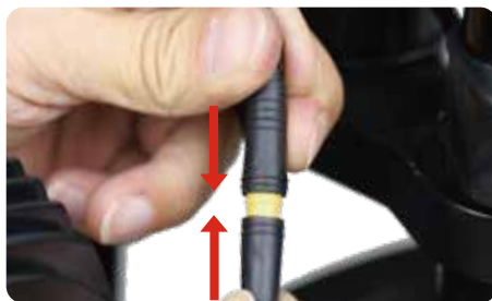
8. Align the combined headlight interface according to the arrow.
