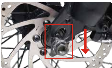
10. Align the bottom opening of the front fork with the front wheel screw and snap it in.
