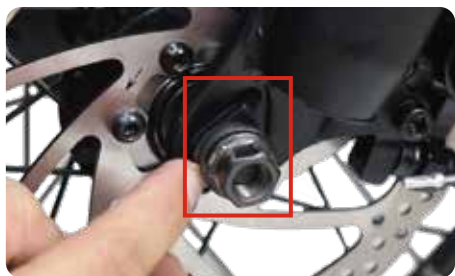
11. Insert the safety hook of the front wheel screw into the safety buckle, and then lock the nuts on both sides.
